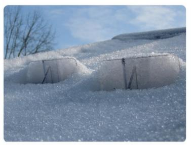
Invented in 1985, the Snojax II is the first "adhesive mounted" clear polycarbonate snow guard. The patented design features unique interchangeable sides that can either be mechanically fastened or adhesive mounted. Use the flat side down on a 5.25" flat surface or simply flip the unit over to straddle a small minor rib. Starter points are provided on both sides for mechanically fastening with self-drilling screws.
