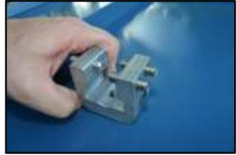
Next, mount the RC-2B bracket on top of the RoofClamp so the large hole in the RC-2B bracket
