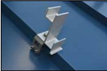
aligns with the threaded hole on top of the RoofClamp. The four smaller holes on the face of the RC-2B bracket will be facing upslope. Use the supplied top bolt and washer to attach the RC-2B bracket onto the RoofClamp using a 9/16" socket. Torque the top bolts to 90 in/lbs. This will be referred hereafter as the RoofClamp/RC-2B assembly.
